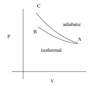
(a) A  $p\alpha = RT$ (a) C  $p_a\alpha_a = RT_a$  where a means adiabatic (a) B  $p_i\alpha_i = RT_i$  where i means isothermal We start at point A and compress a gas either isothermally or adiabatically. Comparing  $\frac{p_a \alpha_a}{p_i \alpha_i} = \frac{RT_a}{RT_i}$ .  $\alpha_a = \alpha_i$  since we need to compare when the gas is compressed to the same volume. Therefore,  $\frac{p_a}{p_i} = \frac{T_a}{T_i}$ .
