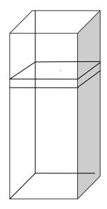
Hydrostatic Equilibrium – surfaces of constant pressure and constant density coincide and are horizontal throughout.
