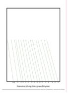
air. They can also be considered to be lines of constant mixing ratio, w, as well. They are labeled at changing interval. Remember if air is lifted dry adiabatically, mixing ratio is conserved (kept constant). If you start lifting air, its initial mixing ratio will not change until the air is lifted to saturation, at which point, the mixing ratio will decrease since vapor is being removed by condensation.
